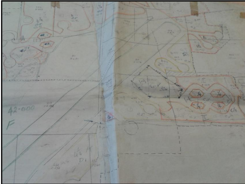
Figure 16: Plans showing the redesign of Hethel at the north-east end of the main runway. The original frying pan has been extended into a spectacle. 35
