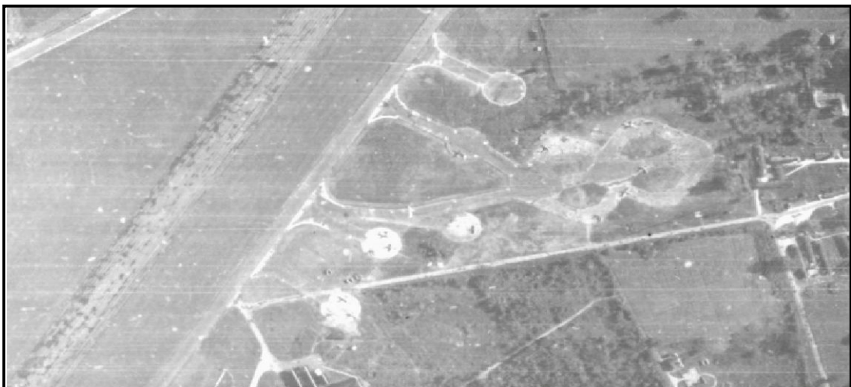
Figure 17: Spectacle stands were introduced after the 'pan' stands to make the airfields more effective as the demands of war increased.
